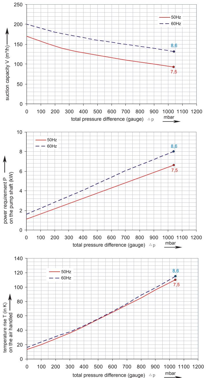
The performance curves are based on air at a temperature of 15 °C and an atmospheric pressure of 1013 mbar with a tolerance of +/- 10 %.
